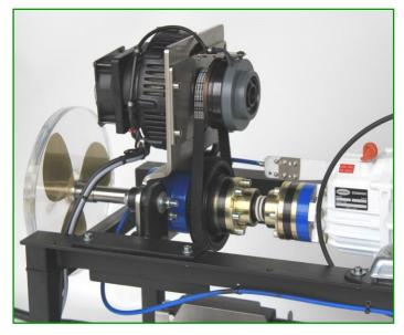
The elsail <u>Hybrid</u> is a so called parallel hybrid; the combustion engine ( diesel or petrol ) and the <u>elsail Hybrid</u> both drive the propeller, but not both at the same time.
